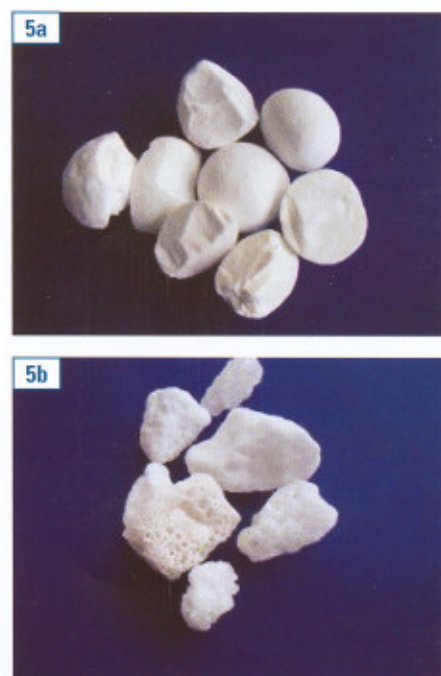
Fig. 5 • Visual appearance of tabular alumina (a) and white fused alumina (b)
