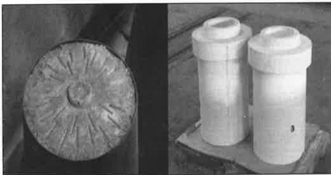
Fig. 6: Application of LC castable with Tabular alumina with AR78 spinel for critical PCPF usages
