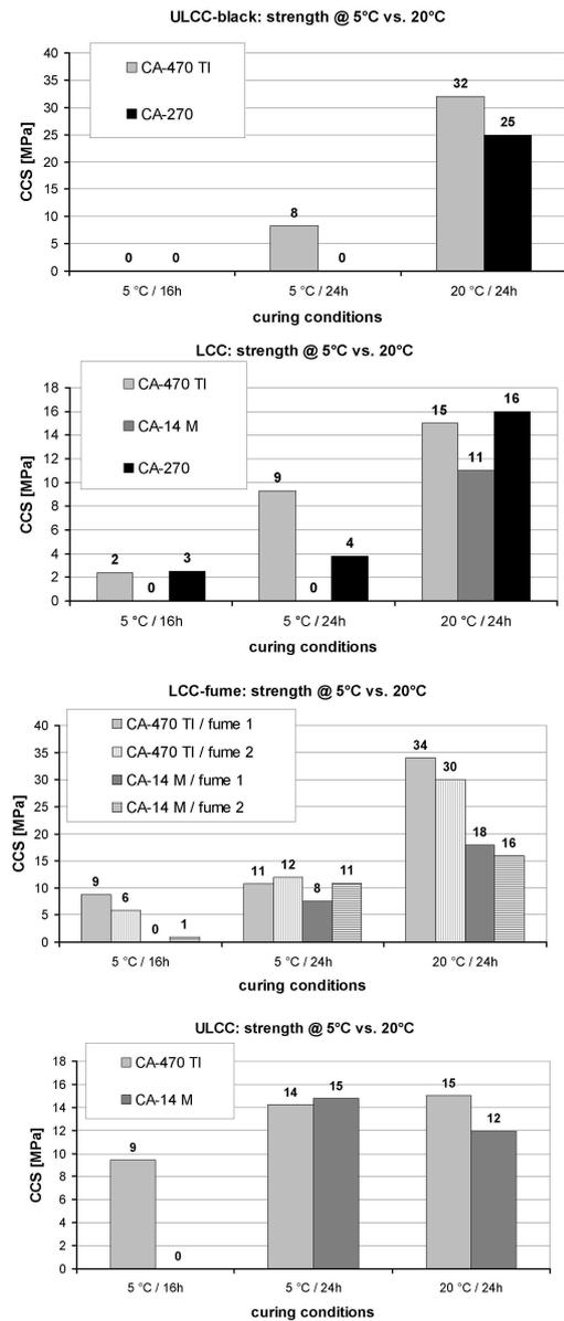
Fig. 4. Cold crushing strength of test castables after curing at 5 and 20 °C. In general lower strength at 5 °C. CA-470 TI showing advantages at low temperatures and in fume containing mixes.
