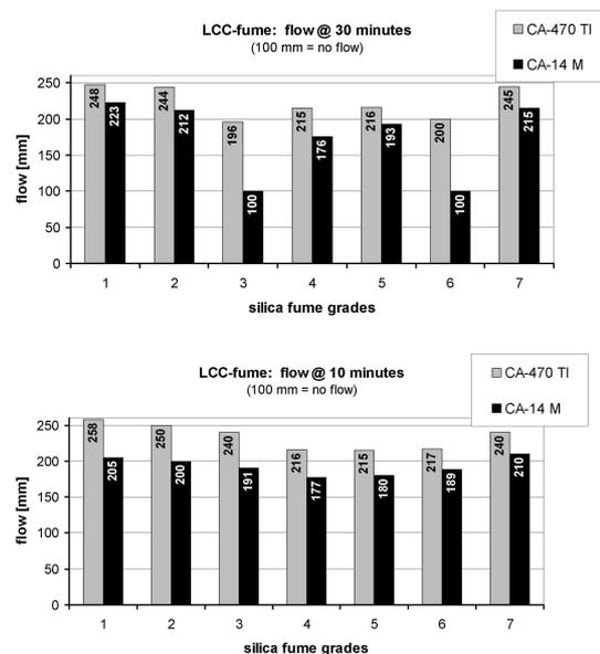
Fig. 5. Self flow data of LCC-fume with different silica fume grades. Tests performed at 5 °C. Better flow values with CA-470 TI.
