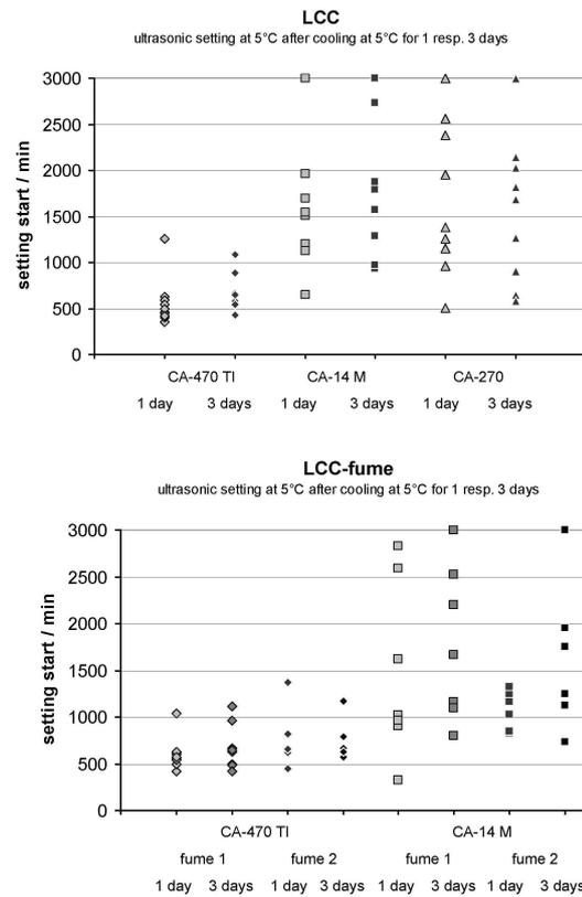
Fig. 1. Repeatability of setting start at 5 °C using ultrasonic equipment. No difference between cooling for one or three days before testing. CA-470 TI shows much more consistent behaviour in repeated testing.
