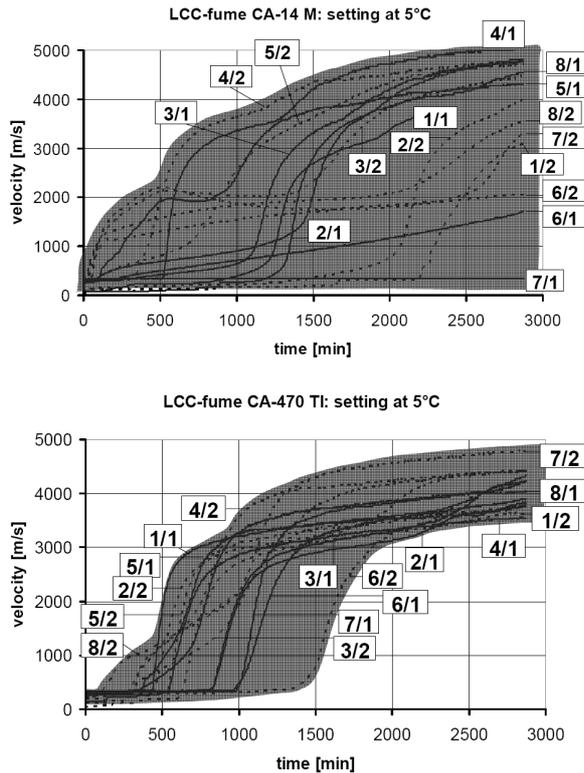
Fig. 2. Ultrasonic setting of LCC-fume with 8 different silica fume grades at 5 °C. Range of setting curves shown by grey background. CA-470 TI shows a more narrow range and no “never setting” behaviour.
