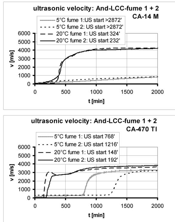
Fig. 3. Setting of Andalusite LCC with silica fume grade 1 and 2 at 5 and 20 °C. Clear advantage of CA-470 TI at 5 °C.
