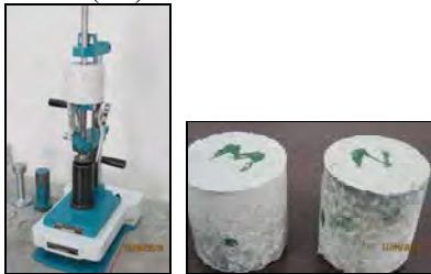
Fig 14 Rammed cylinder (right) preparation by sand rammer (left)
