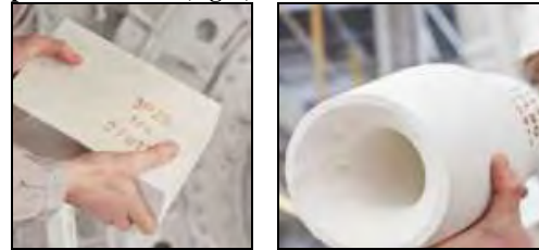
Fig. 5 Typical application of tabular alumina containing products: corundum bricks (left), pressed nozzles (right)
