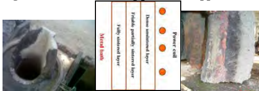
Fig 19 Controlled sintering pattern in application
