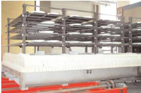
Fig. 8 Kiln car for the glost-firing porcelain kiln
