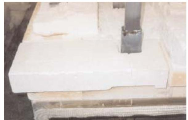
**Fig. 5** The new material offers complex geometry: cornerstones in the support area
