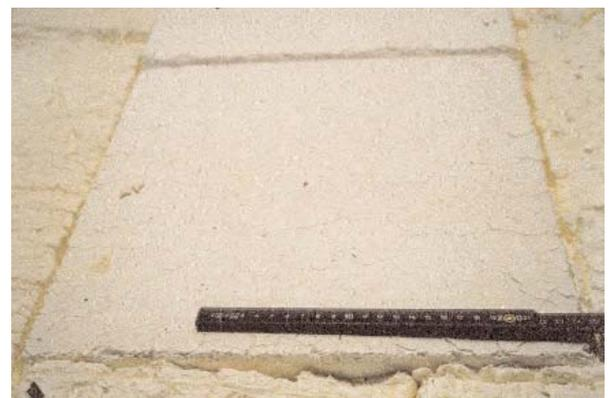
**Fig. 6** Hardly any cracks: network of cracks on the SiO<sub>2</sub>-containing brick
