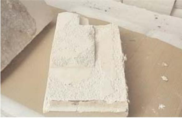
Fig. 7 Excellent binding: the new microporous refractory material with lightweight refractory bricks
