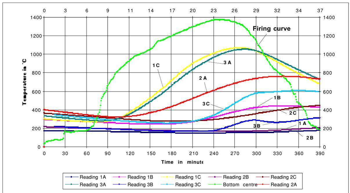
Fig. 9 Temperature readings from a kiln car with different thermal insulation systems
