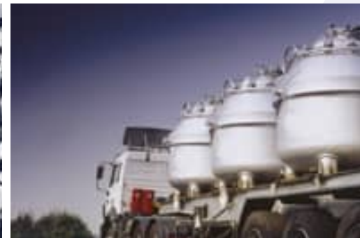
APPLICATION: Liquid aluminum transport
