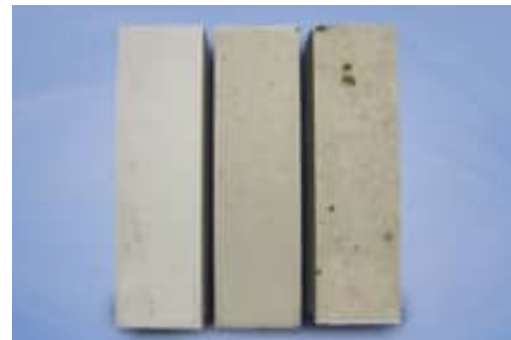
BSA 96 (middle) shows no melt-outs compared to BFA (right); tabular alumina (left) for comparison
