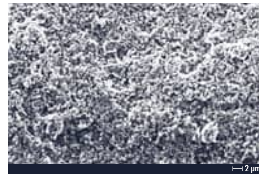
Reactive alumina RG 4000 fully ground to primary crystal
