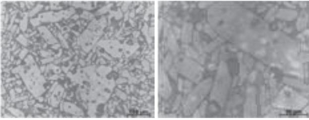
Fig. 3: SEM micrographs of BSA 96 grain; thermally etched at 1500°C
