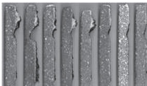
Fig. 5: Cut sections of AMC bricks after induction furnace test at 1650 °C and average wear rate at slag level in mm/h.
