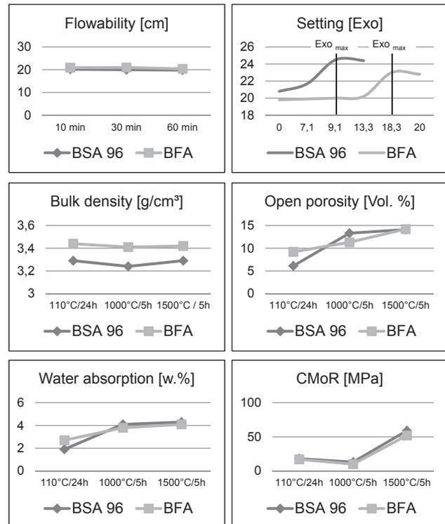
Fig. 4: Comparison of physical properties of BSA 96- and BFA-based LC-castables
