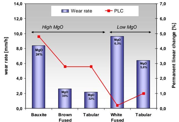
Fig. 9: Induction furnace slag test at 1650 °C / 2 h and CaO:Al<sub>2</sub>O<sub>3</sub> ratio = 1.08 (+ CaF<sub>2</sub>). Resin bonded AluMagCarbon bricks with high and low MgO content. Permanent linear change is considerably higher with high MgO content
