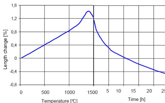
Fig. 7: Creep resistance of dense calcium hexaluminate, Bonite, based castable after pre-firing at 1500 °C / 5 h
