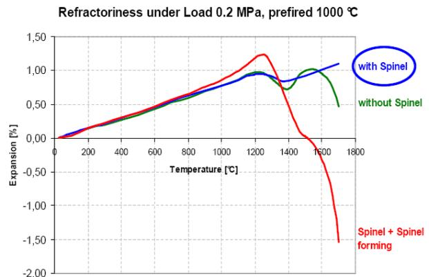
Fig. 10: Refractoriness under load (RuL) of tabular and spinel self flowing castables (samples pre-fired 1000 °C / 5 h)
