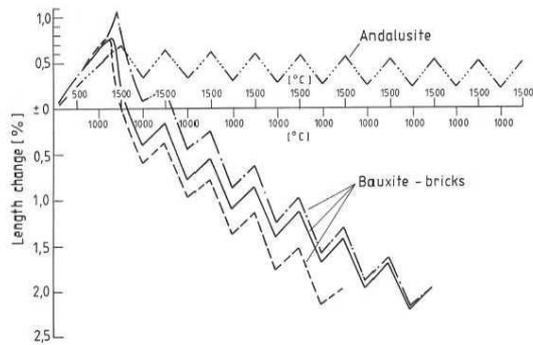
Fig. 4: Creep of andalusite and bauxite bricks tested under torpedo car application conditions; load 0.2 MPa, temperature change between 1000 and 1500 °C [27]
