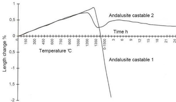
Fig. 12: Creep resistance of Andalusite based low cement castables at 1500 °C. Castable 2 with matrix aluminas (HCS at 1500 °C: 11 MPa), castable 1 without (HCS 1 MPa) [30]
