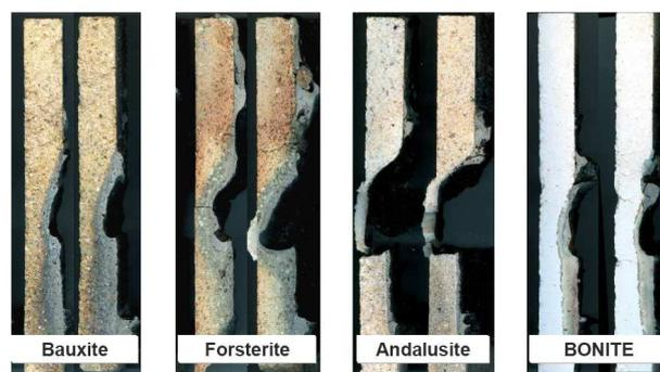
Fig. 6: Induction furnace slag test at 1600 °C / 2 h and CaO:Al<sub>2</sub>O<sub>3</sub> ratio = 1.08. Bricks of Andalusite, Bauxite, Forsterite vs. Bonite (dense CA<sub>6</sub>) castable [24]
