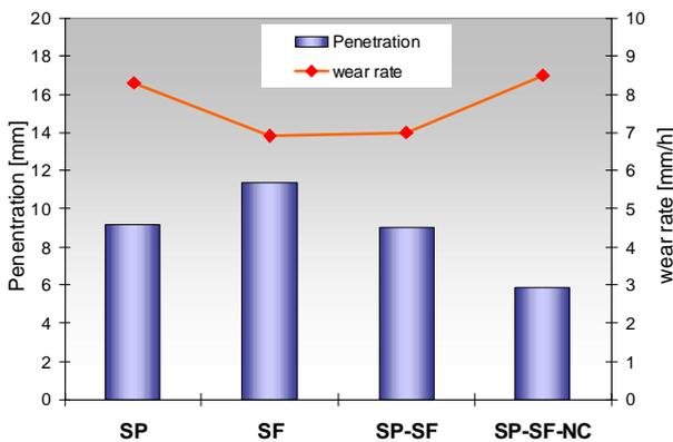
Fig. 8: Induction furnace slag test at 1650 °C / 2 h and CaO:Al<sub>2</sub>O<sub>3</sub> ratio = 1.08 (+ CaF<sub>2</sub>). Spinel (SP) and Spinel forming (SF) castables and combinations thereof; MgO contents between 4.5 and 6.3 %, open porosity at 1500 °C between 15.3 and 17.7 % [35]
