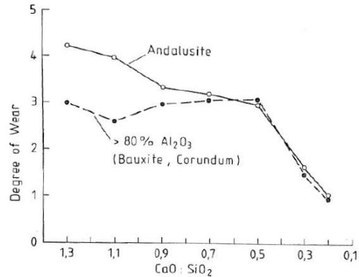
Fig. 3: Resistance of andalusite and bauxite / corundum bricks against slag with different  $CaO:SiO_2$  ratio at 1520 °C / 4 h [27]
