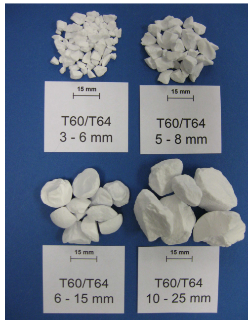
Fig. 1. Coarse sizes of tabular alumina T60/T64.
