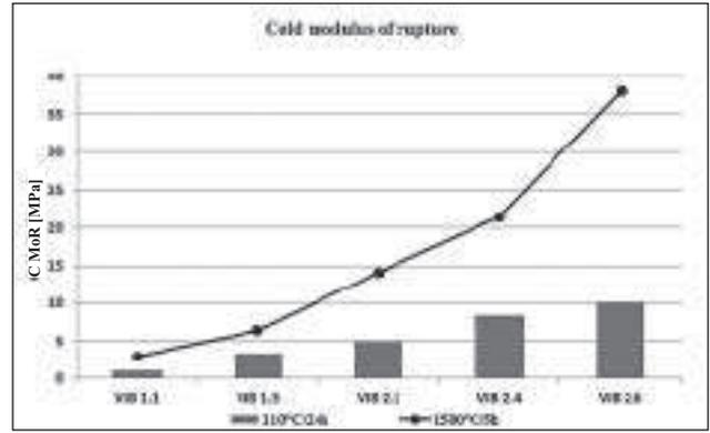
Fig. 4: Cold modulus of rupture of CA<sub>6</sub> based vibration castables
