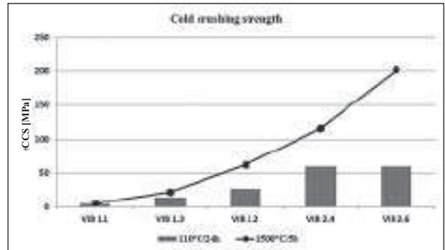
Fig. 5: Cold crushing strength of CA<sub>6</sub> based vibration castables
