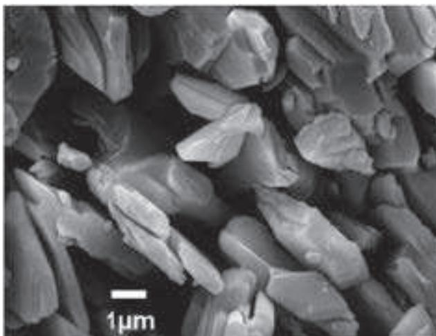
Fig. 1: Microstructure of lightweight  $CA_6$  SLA-92
