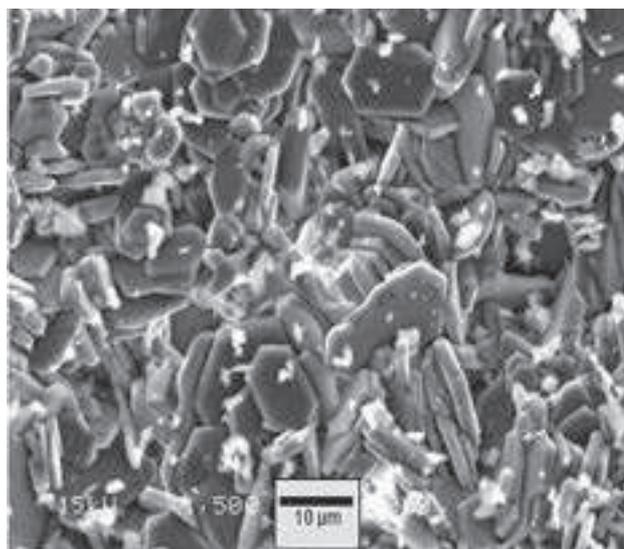
Fig. 2: Microstructure of dense  $CA_6$  Bonite (different scale to be considered compared to figure 1)
