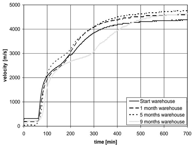
Fig. 2b. Ultrasonic graphs of LCC-ADS/W / warehouse storage
