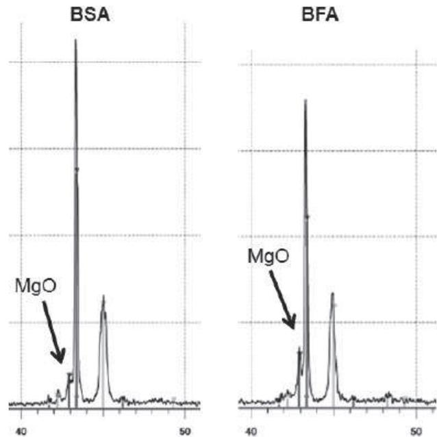
Fig. 2: XRD of AMC bricks BSA and BFA after 1500°C / 5 h reducing conditions; different periclase (MgO) peak height.
