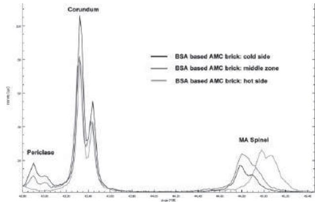
Fig. 7: Temperature dependent formation of Spinel in BSA based AMC brick from the ladle side wall trial.
