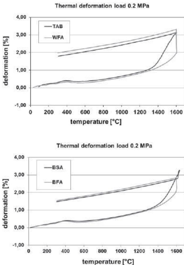
Fig. 6: Dilatation of AMC bricks in reducing condition, load 0.2 MPa, 6 h holding time at 1600°C; TAB and WFA (up); BSA and BFA (down).
