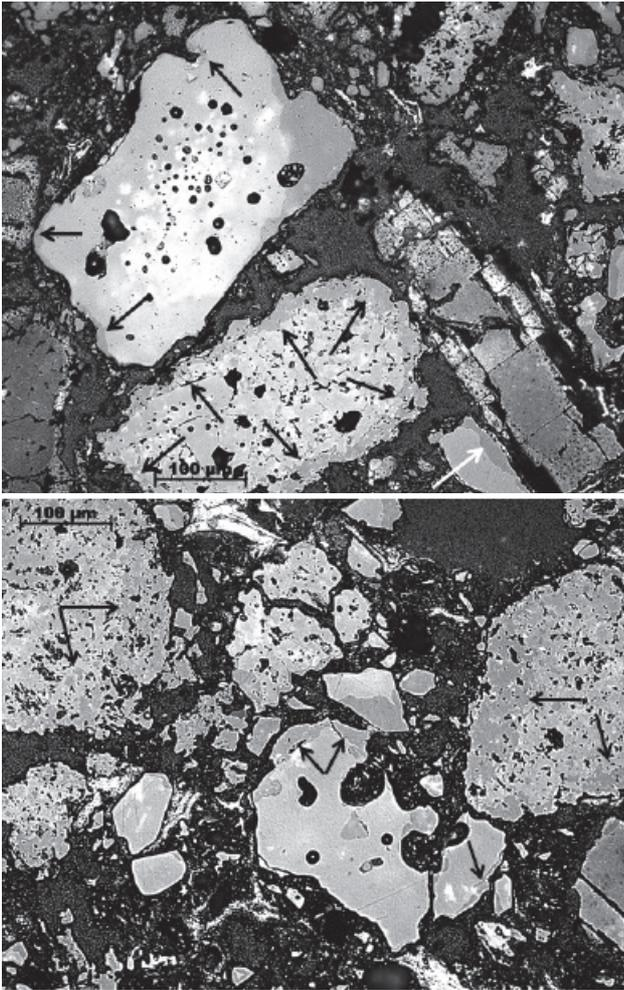
Fig. 3: Reflected light microscopy of BSA 96 and BFA grains in AMC brick fired 5 h in reducing condition at 1400 °C (up; periclase grains in lower left and right corner) and 1500 °C (down), see text.
