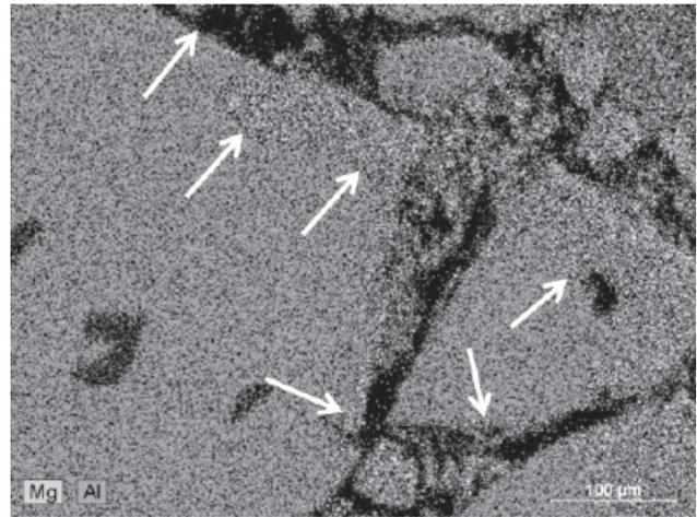
Fig. 4: EDX of BSA 96 (up) and BFA (down) grains in AMC brick fired at 1600 °C / 5 h in reducing conditions.
