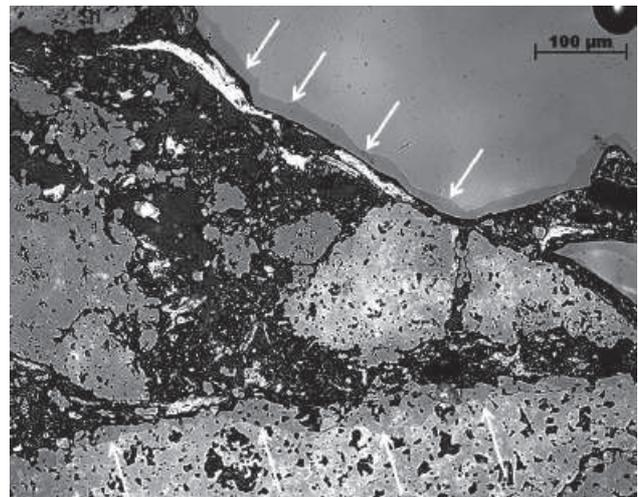
Fig. 5: Reflected light microscopy of TAB and WFA grains in AMC brick fired at 1600 °C / 5 h in reducing conditions.
