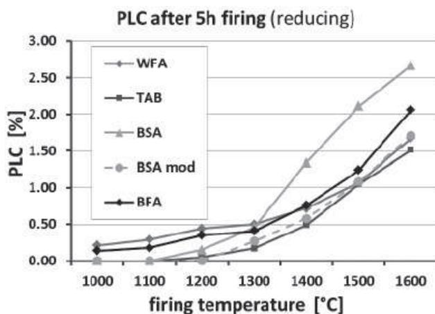
Fig. 1: Permanent linear change of AMC bricks, fired under reducing conditions for 5 hours.
